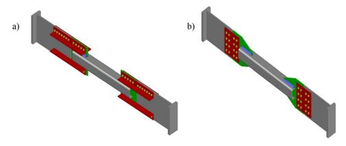
Figure 11. Paddle-gusset plate connection scenarios; a) 4-Angle, and b) 2-Plate.
