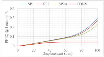
Figure 5. PEEQ at location B vs. Displacement for different overlap lengths.
