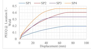
Figure 10. PEEQ at location E vs. Displacement at weld tip for different overlap lengths.
