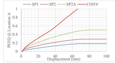
Figure 4. PEEQ at location A vs. Displacement for different overlap lengths.
