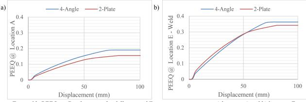
Figure 13. PEEQ vs. Displacement for different paddle-gusset connections at a) location A and b) location E.
