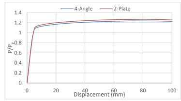
Figure 12. Global load-displacement for different paddle-gusset connection scenarios.
