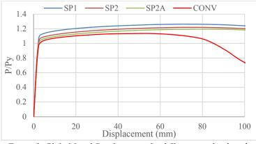
Figure 3. Global Load-Displacement for different overlap lengths.
