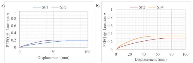
Figure 9. PEEQ at location A vs. Displacement at location A for a) Lwg=20mm and b) Lwg=10mm.
