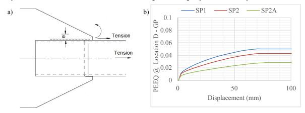
Figure 6. a) SHG connection detail showing flexural demand, b) PEEQ at location D vs. Displacement for different overlaps.
