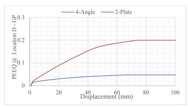
Figure 14. PEEQ at location D vs. Displacement for different paddle-gusset connections at slot of gusset plate.
