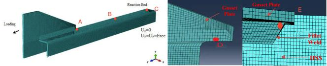
Figure 2. FE Model Showing mesh, boundary conditions, and locations of evaluation.
