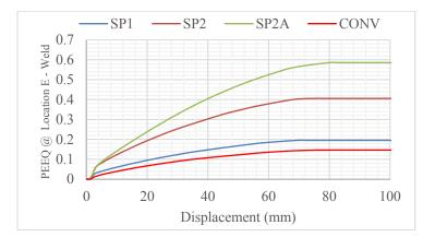
Figure 7- PEEQ at location E vs. Displacement for different overlap lengths.
