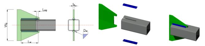
Figure 1. Details of SHG HSS brace connection and assembly of parts.
